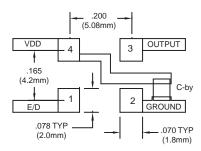
Bypass capacitor. C-by, should be
